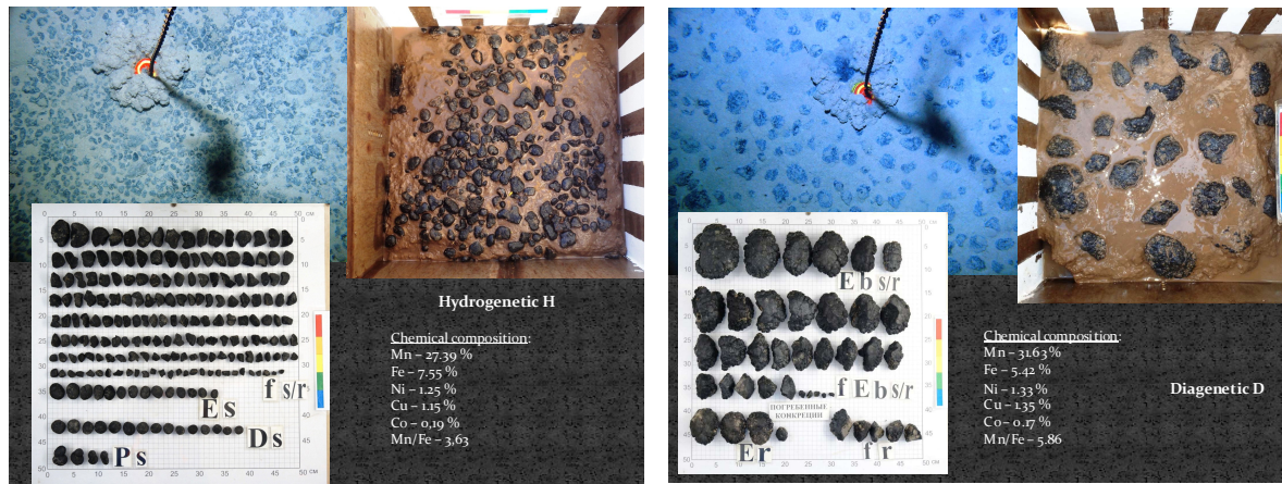
Fig.8. Box corer sampling with hydrogenetic (left) and diagenetic (right) nodules.
