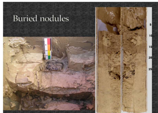
Fig.9. Buried nodules in box corer found at the depths 20-25 cm.
