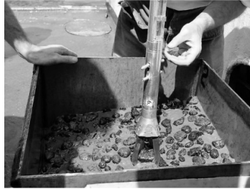
Fig. 2 A special device for rip off force measurements
