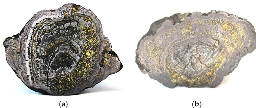
Figure 3. Example views of the chipping (a) and smooth (b) cross-sections of polymetallic concretions formed using a high-pressure AWJ.
