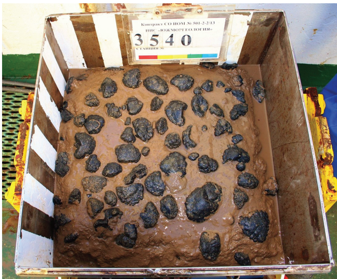
Fig. 7. Collected box-corer sample of sediment with polymetallic nodules after draining the water
