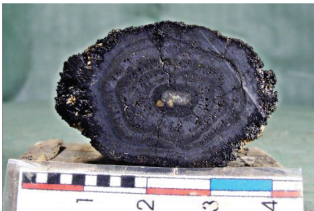
Fig. 10. Internal structure of polymetallic nodule
